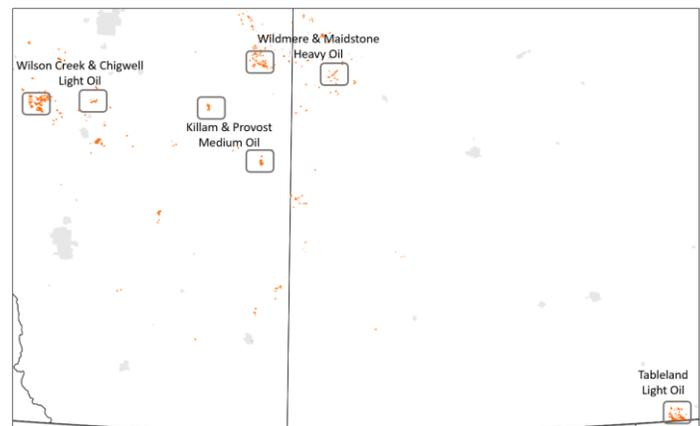
The core areas that are currently (or planned to be) under flood through the next couple months are highlighted in the above map. Interestingly, the combined total production from all the planned water flood patterns is about 675 boes per day or approximately 11 per cent of Gear's total current production. With future investment we will continue to expand that percentage and work toward our goals of an extending Gear's reserves life, and continuing to shallow the corporate base decline.
